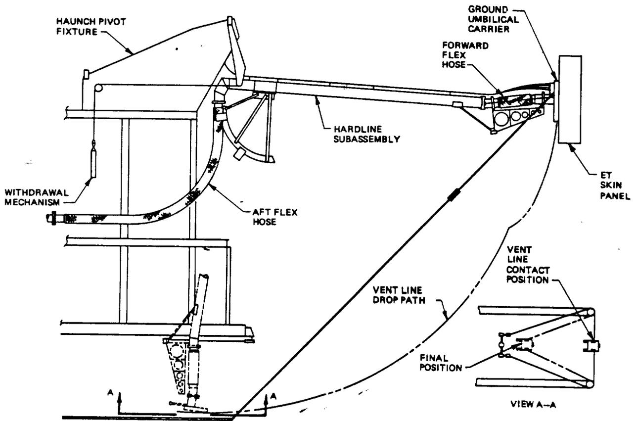
FIGURE 4. ET HYDROGEN VENT UMBILICAL SYSTEM
