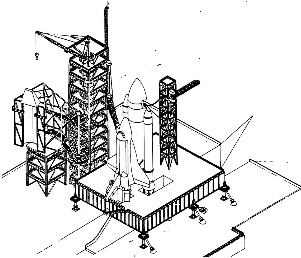
FIGURE 2.  $\text{GH}_2$  VENT LINE CONCEPT II (TOWER ON MLP)
