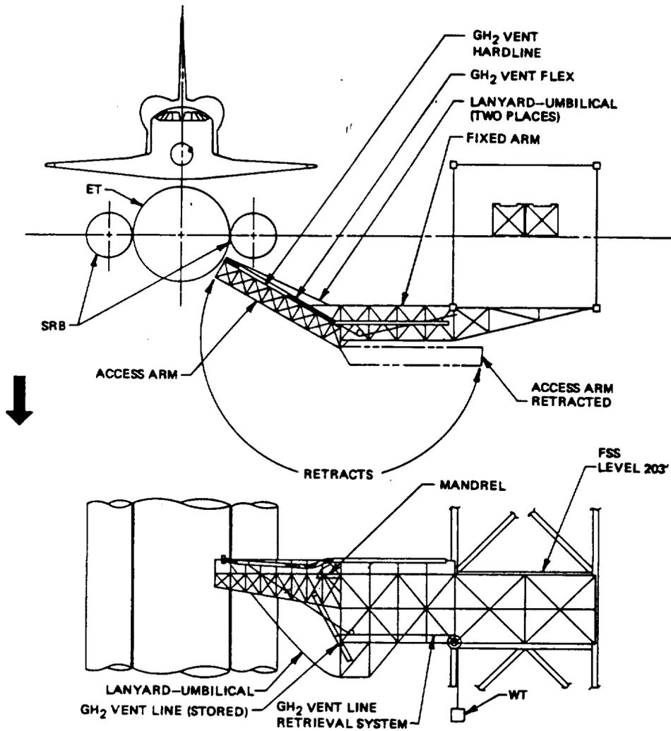
FIGURE 3. GH<sub>2</sub> VENT CONCEPT III (BASE FROM FSS)
